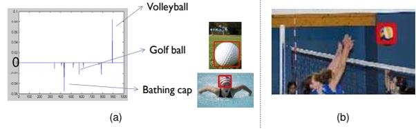
Figure 10. The weights of image classification scores (a) for the object detection class volleyball (b).
